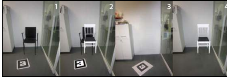
Figure 1.4.. An example of a diminished reality technique in AR. 1. Original visual 2. AR process on existing object 3. Implementation of the diminished reality technique. 4. Implementation of AR on diminished reality (Siltanen, 2012).
